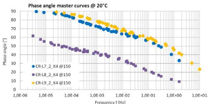
Figure 6 Phase angle master curve for CRmBs with pulverized rubber of different grading
