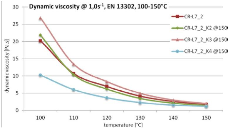
Figure 1 Flow (viscosity) curves for CRmBs with different catalysts
