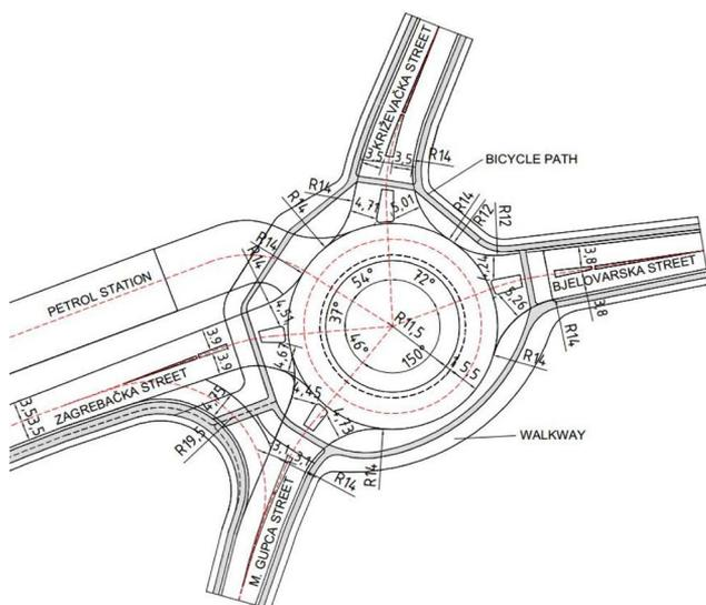
Figure 1 Plan of the roundabout in Vrbovec
