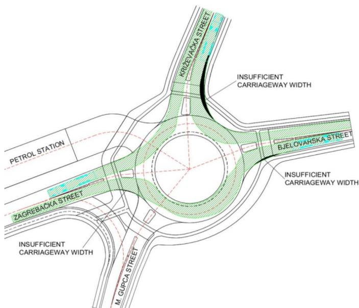
Figure 3 Offtracking control of the roundabout in Vrbovec
