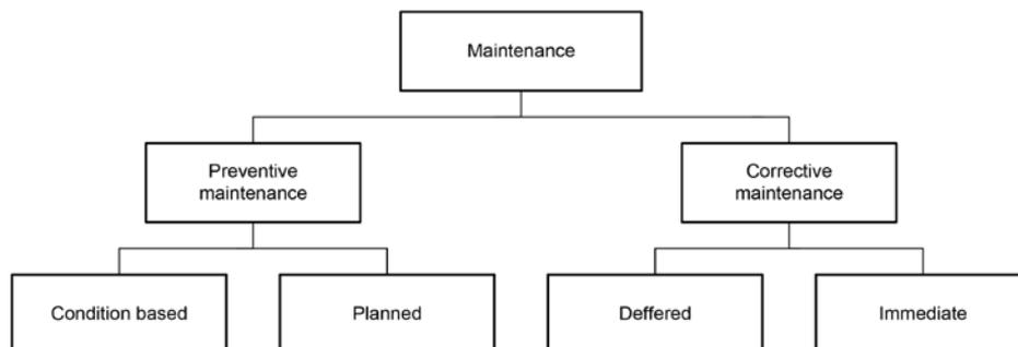
Figure 2 Types of maintenance of railway track [3]
