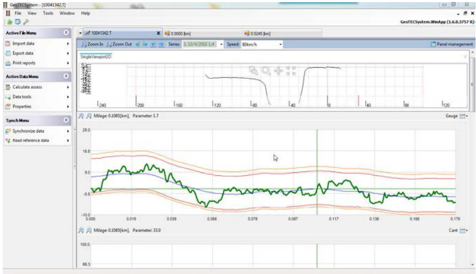
Figure 3 Exemplary track geometry and rail head measurement results
