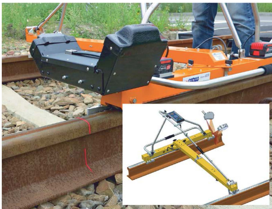
Figure 2 Track geometry and rail head profile trolley
