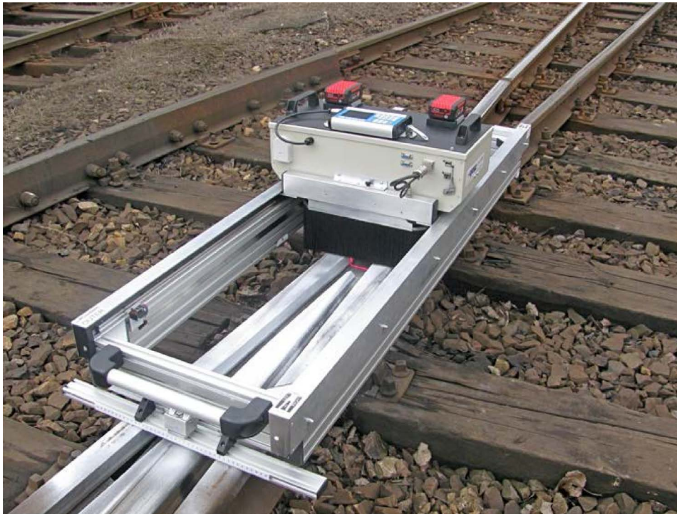
Figure 6 Optical system for track and turnout measurement
