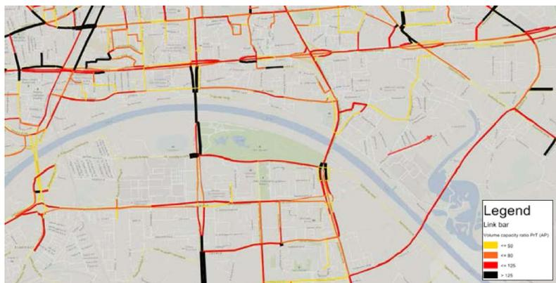
Figure 6 Saturation of proposed network in year 2033
