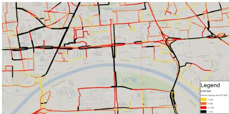
Figure 5 Saturation of the network in year 2033 (Scenario 2033\_V1-0)
