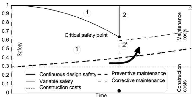
Figure 3 Time related connection between maintenance cost and safety level
