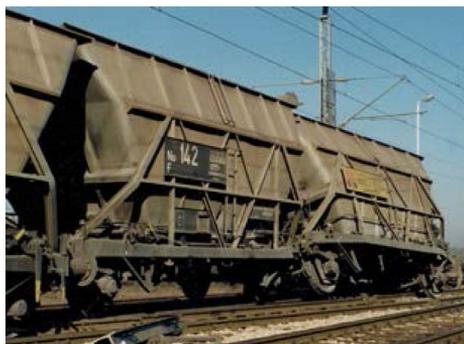
Figure 1 The derailment caused by the failure of the suspension system
