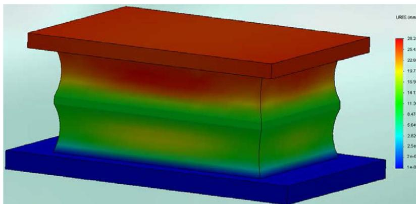
Figure 8 The deflection of rubber-metal elastic element
