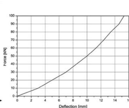
Figure 7 The diagram of stiffness of finally adopted rubber-metal element
