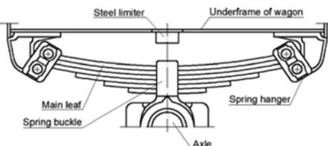
Figure 2 The scheme of suspension of Fbd wagon
