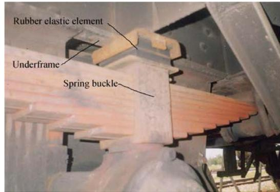
Figure 5 The rubber-metal elastic element instaled in suspension
