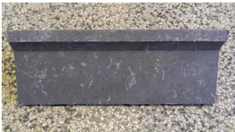
**Figure 4** Plastic sleeper anchor after abrasion resistance test
