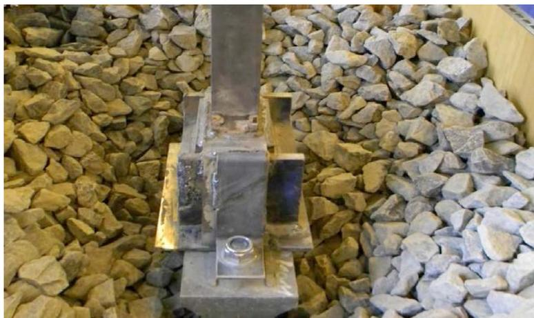
**Figure 3** Test of tearing resistance in ballast
