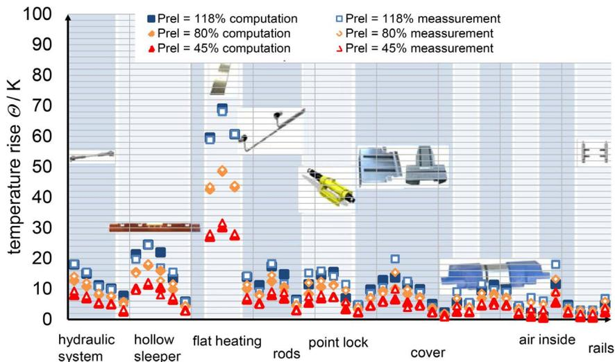
Figure 3 Experimental verification of thermal network with open apertures
