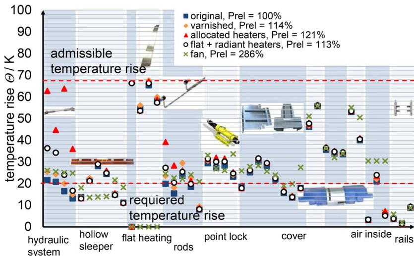
Figure 4 Computed temperature distribution for various designs of the heating system
