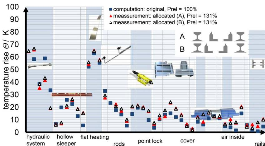
Figure 5 Experimental temperature rise with several allocated heating elements
