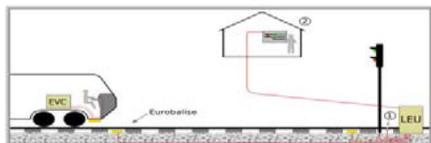
Figure 2 Schematic diagram of ETCS – Level 1[1]
