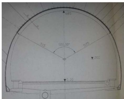
**Figure 4** Support systems of the main tunnel – type III
