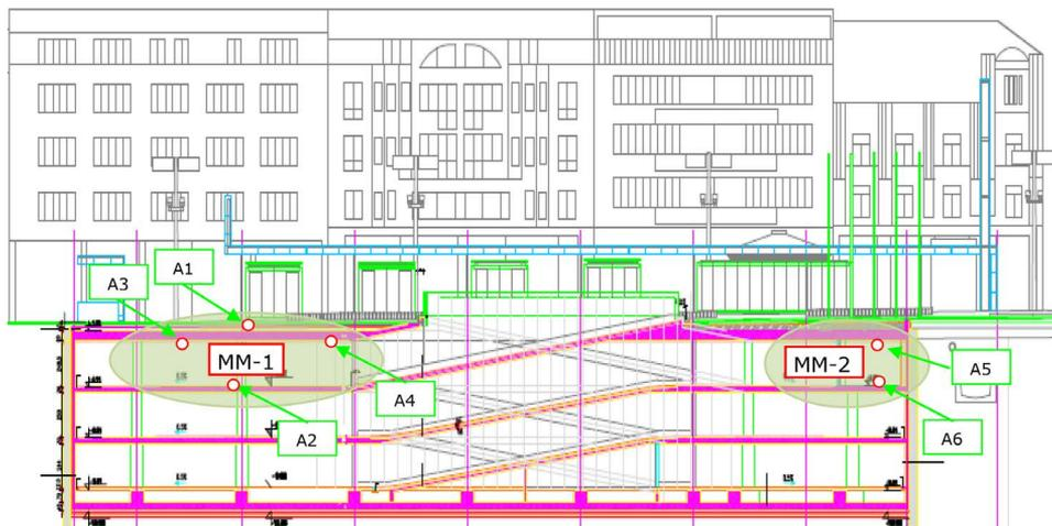
Figure 3 Kvaternik square garage cross-section with measuring locations
