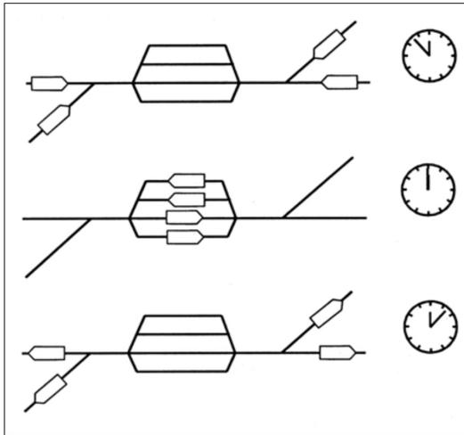
Figure 1 Basic principle of an integrated timetable
