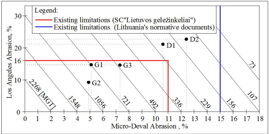
Figure 2 Lifespan prognostic graphic model of ballast aggregate as sleepers are made of concrete
