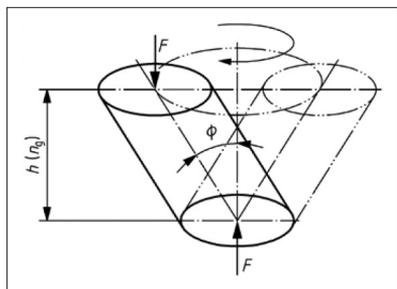
Figure 1 Sample motion diagram at gyrator compaction
