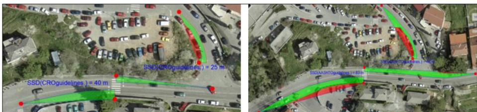
**Figure 3** Sight triangle visualisations for pedestrian crossings on major and minor road considering calculated stopping sight distance using Croatian guidelines (left scheme) and AASHTO's Greenbook (right scheme)
