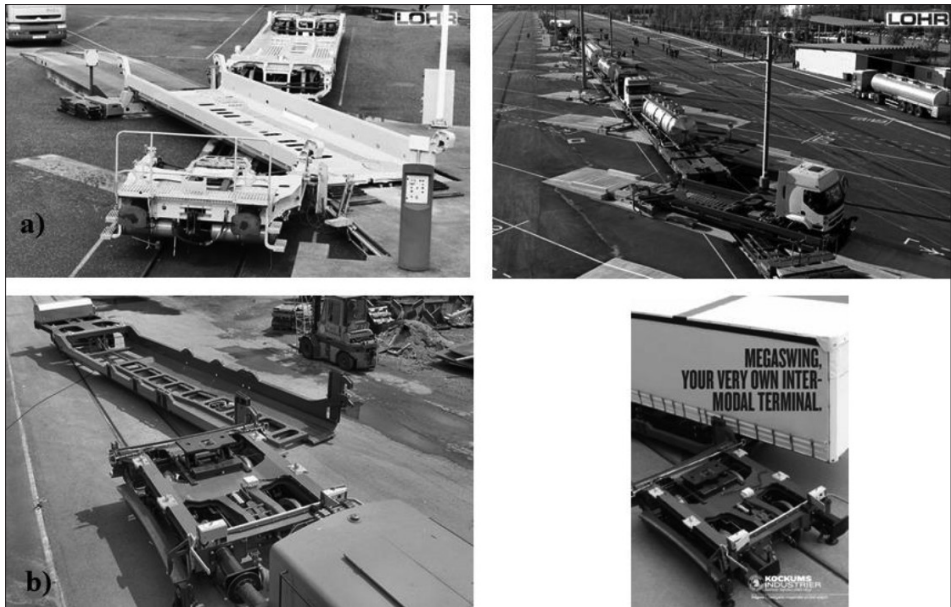
Figure 1 Wagons for trucks semitrailers transportation: a) developed by French company Moda Lohr [2], b) Megaswing developed by Swedish company Kockums Industrier [3].
