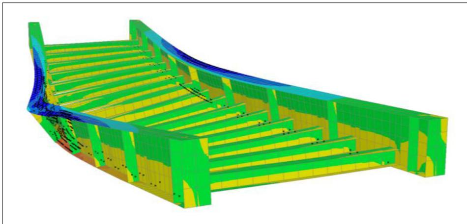
**Figure 4** Buckling with yielding, from nonlinear analysis of U-frame deck
