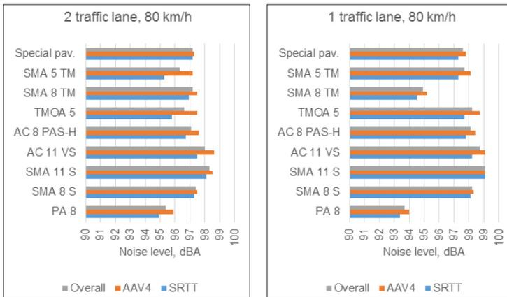
Figure 4 CPX noise level on both lanes at 80 km/h speed
