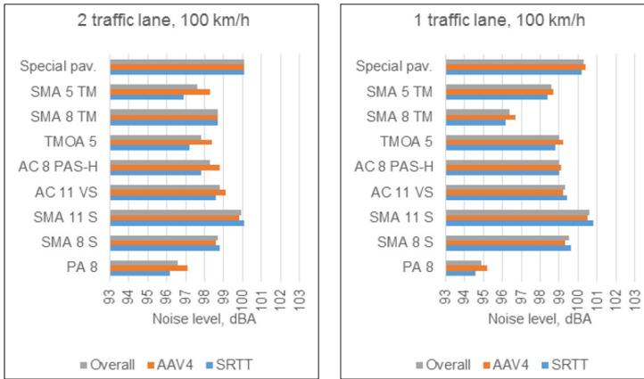
Figure 5 CPX noise level on both lanes at 100 km/h speed
