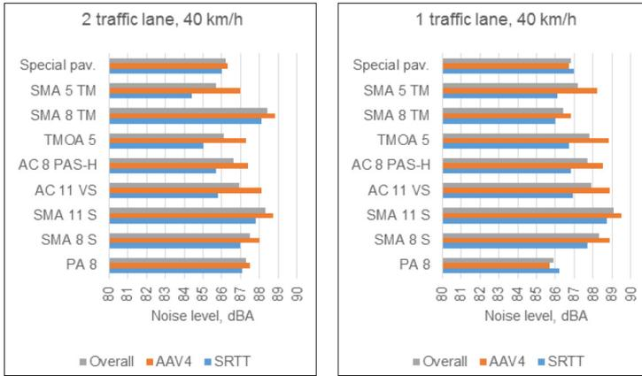
Figure 2 CPX noise level on both lanes at 40 km/h speed
