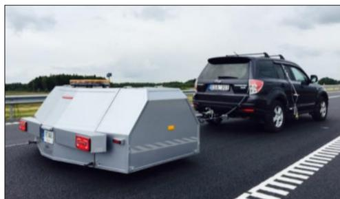
**Figure 1** Fragment from CPX noise level measurements
