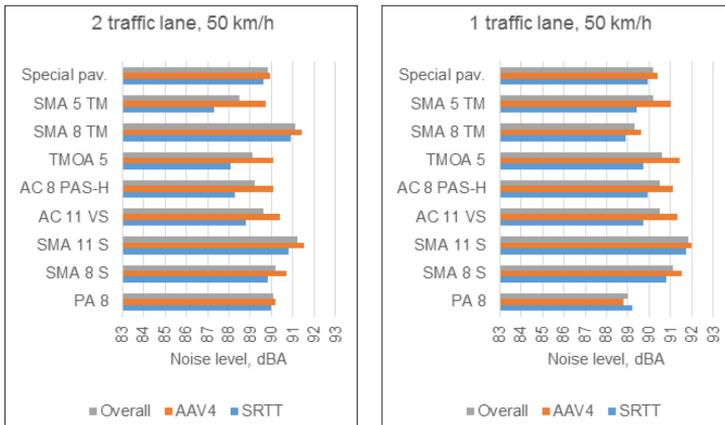
Figure 3 CPX noise level on both lanes at 50 km/h speed
