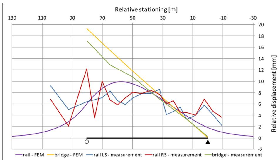
Figure 4 Example of displacements evaluation, bridge No. 2
