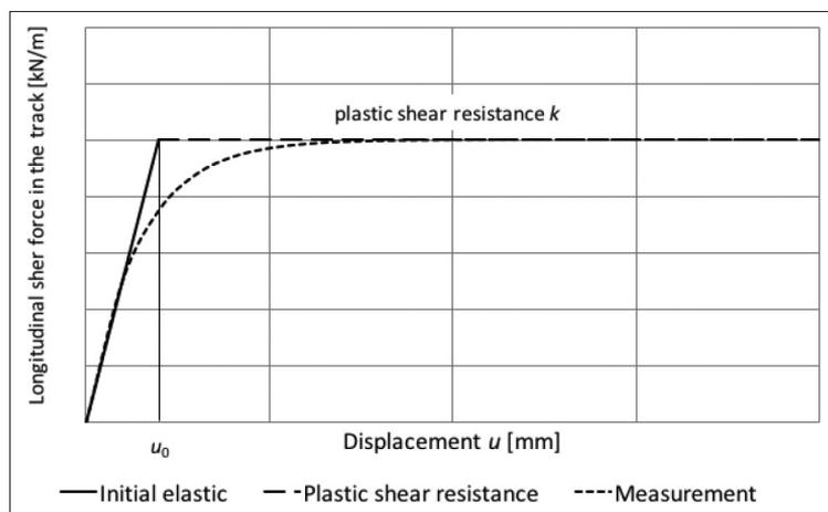
**Figure 2** Variation of longitudinal shear force with longitudinal track displacement
