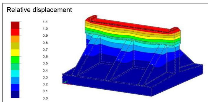
**Figure 1** FEM analysis of the steel bridge bearing
