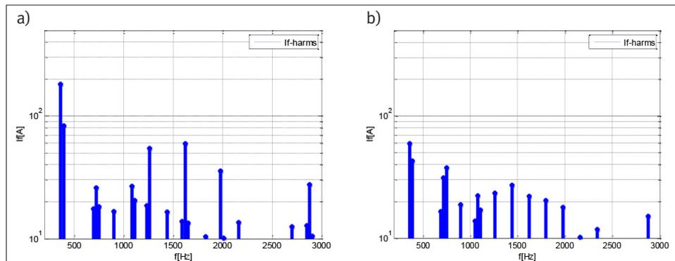
**Figure 3** Results of simulation calculations of DC-link current harmonics generated by a 0.5 MW drive system: a) full power; b) reduced power
