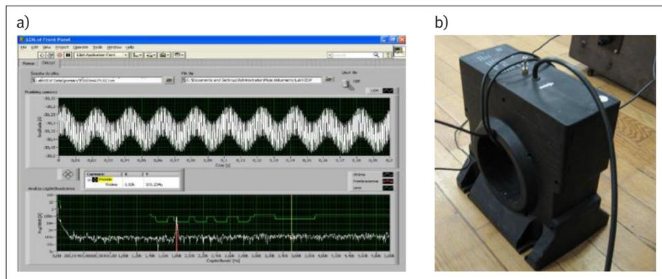
**Figure 2** The elements of a laboratory model of the system used for on-line monitoring of the harmonics in current consumed by a converter from a DC network: a) a screenshot of an application developed in the LABVIEW environment; b) LEM RA 2000-S/SP1 converter.
