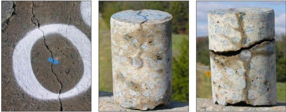
**Figure 1** Vertical crack on the surface of a bridge deck (left), a core with a vertical crack (middle), and a core with a vertical crack and delamination (right)
