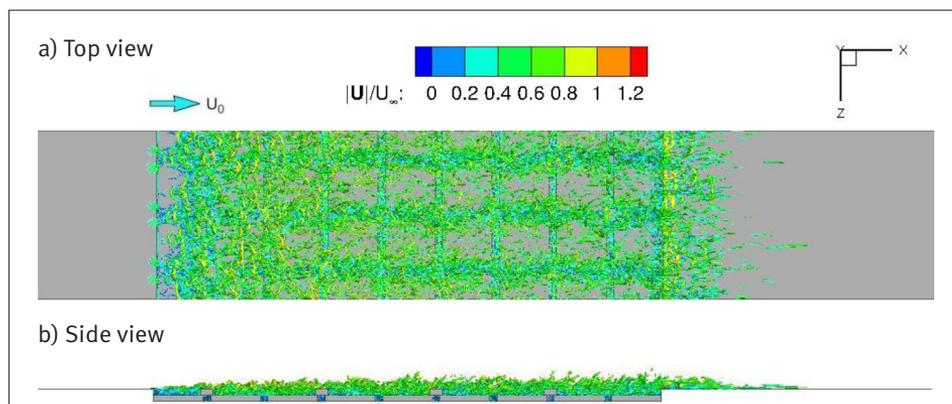
**Figure 2** Iso-surfaces of the instantaneous normalized Q-criterion
