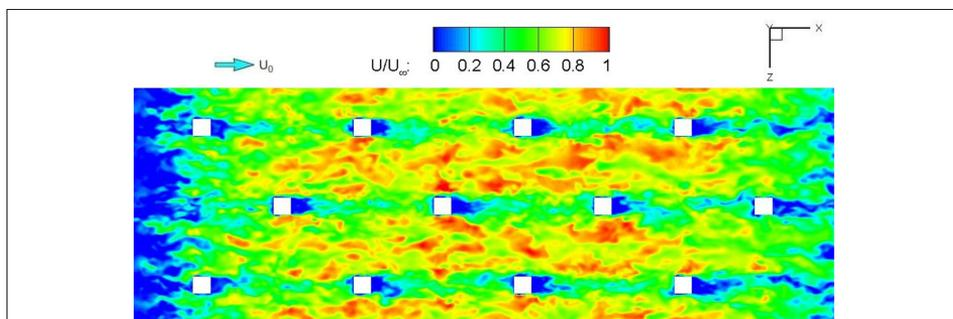
Figure 5 Contours of instantaneous velocity through the ballast particle horizontal mid-plane (top view)
