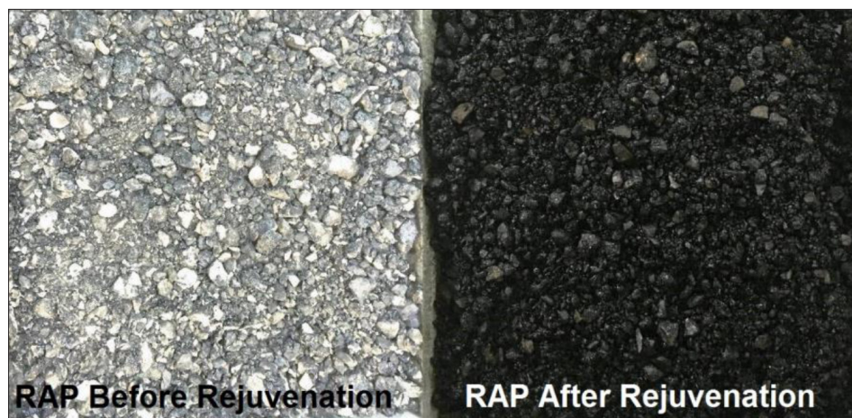
Figure 1 RAP before and after rejuvenation with WEO
