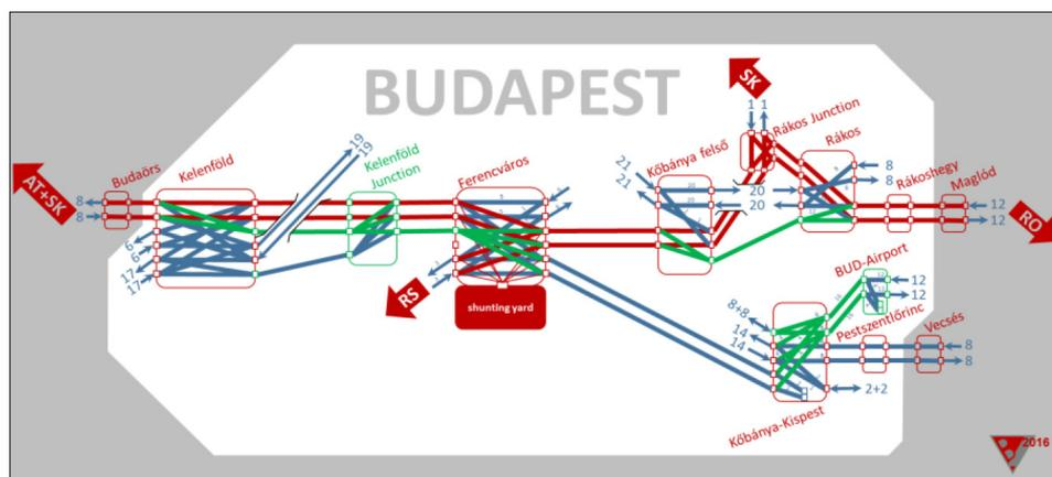
Figure 5 This figure shows the routes of cargo trains (red), all proposed new tracks (green) and the routes and number of passenger trains in a two hours period (blue)
