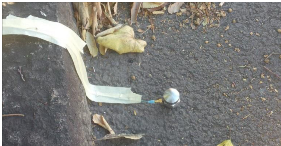
Figure 17 Placements of an accelerometer
