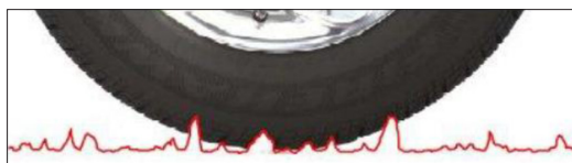
Figure 2 Positive texture of the road surface
