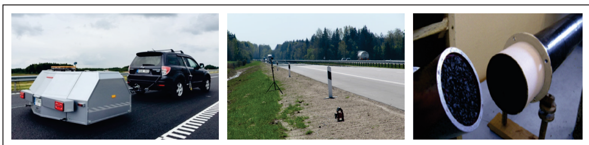
Figure 1 Fragment from CPX (left), SPB (middle), Standing wave tube (right) noise level measurement
