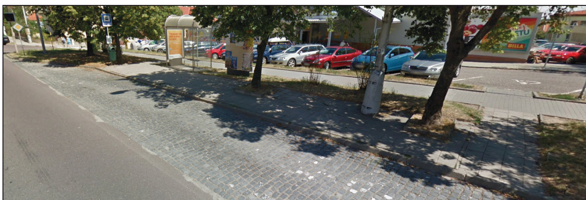
Figure 3 An example of an inappropriate solution of the entrance area – the bus stop curb is missing and also the contrast signs of the entrance edge including the signal strip. In the area of the platform there are obstacles for the pedestrians. There is also a pedestrian crossing at the beginning of the entrance area.
