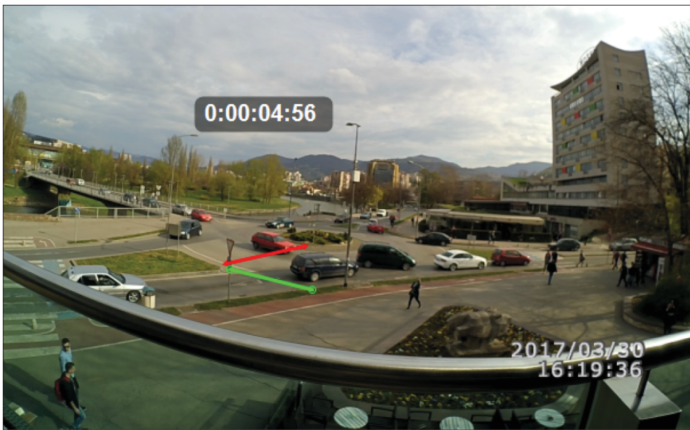
Figure 2 Video recording of single-lane roundabout “Evropa” and extracting gap values
