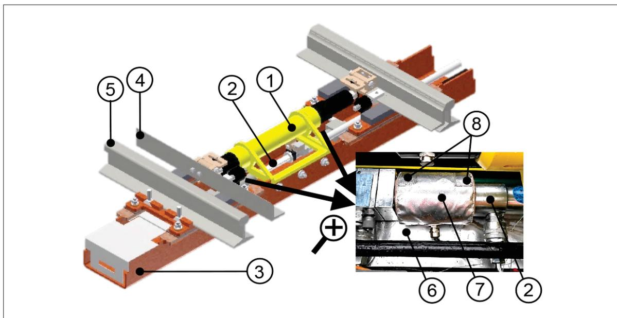
Figure 1 Optimised heating system with two heating jackets and a flat heater
