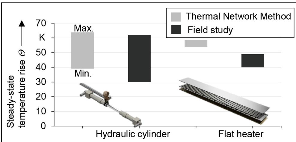
Figure 6 Maximum and minimum steady-state temperature rise of critical components previously computed with Thermal Network Method [1] and now measured during field study
