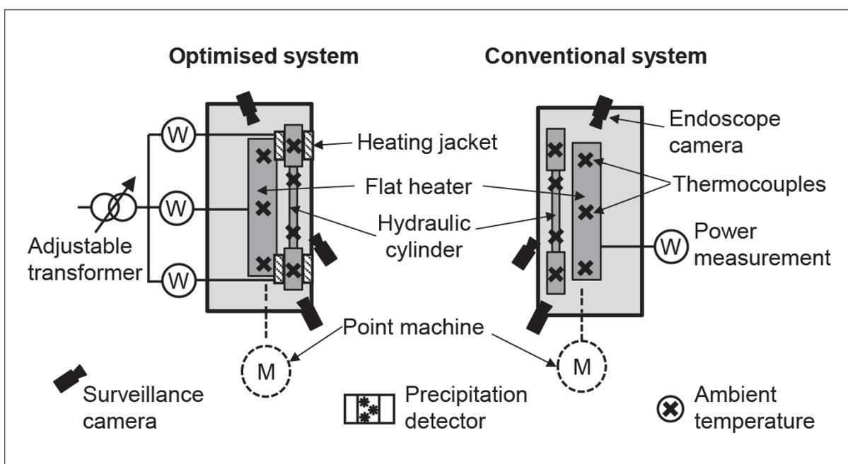
Figure 3 Experimental set-up of the optimised system and the conventional sys. at the high-speed railway line
