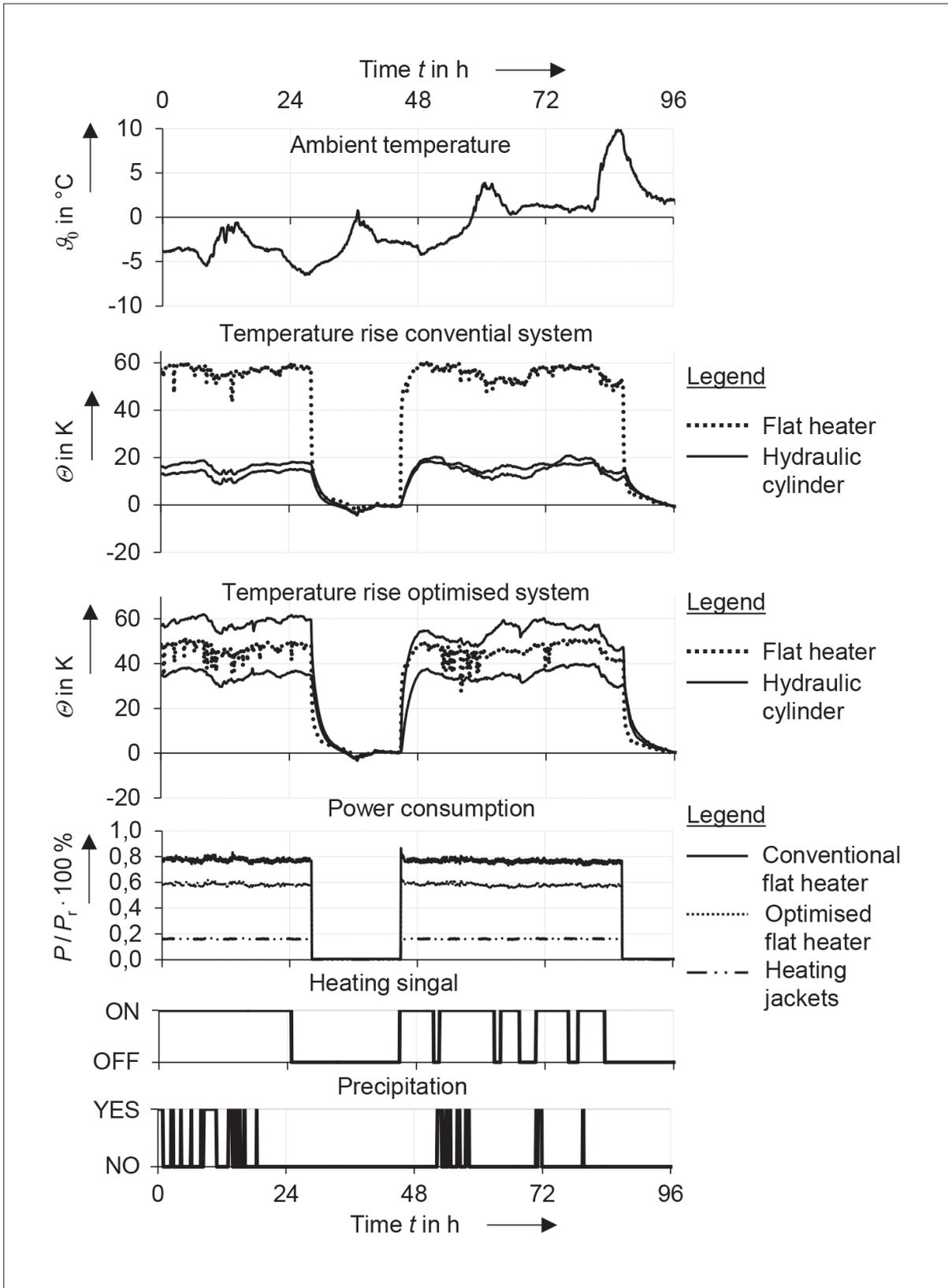
**Figure 4** Recorded sequences of ambient temperature, critical temperature rises and power consumption of the conventional system and optimised system, heating status and precipitation, starting at 12.00 a.m. on 5<sup>th</sup> January 2016
