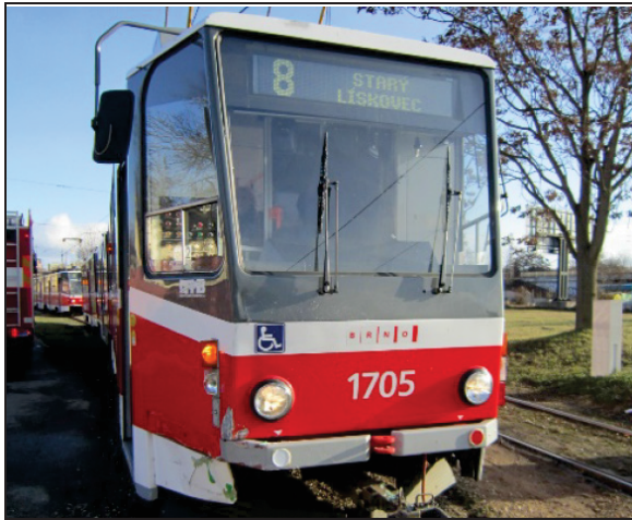
Figure 3 Left: the nose of a tram with a coupler (accident No. 5); right: the nose of a modern tram without a coupler (accident No. 6)
