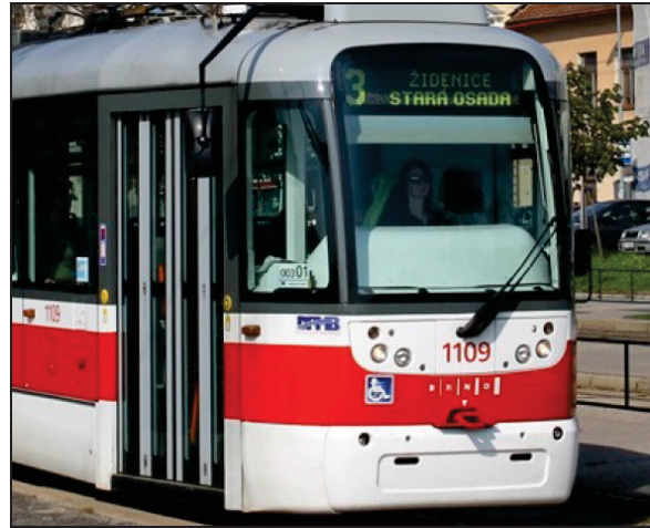
Figure 3 Left: the nose of a tram with a coupler (accident No. 5); right: the nose of a modern tram without a coupler (accident No. 6)
