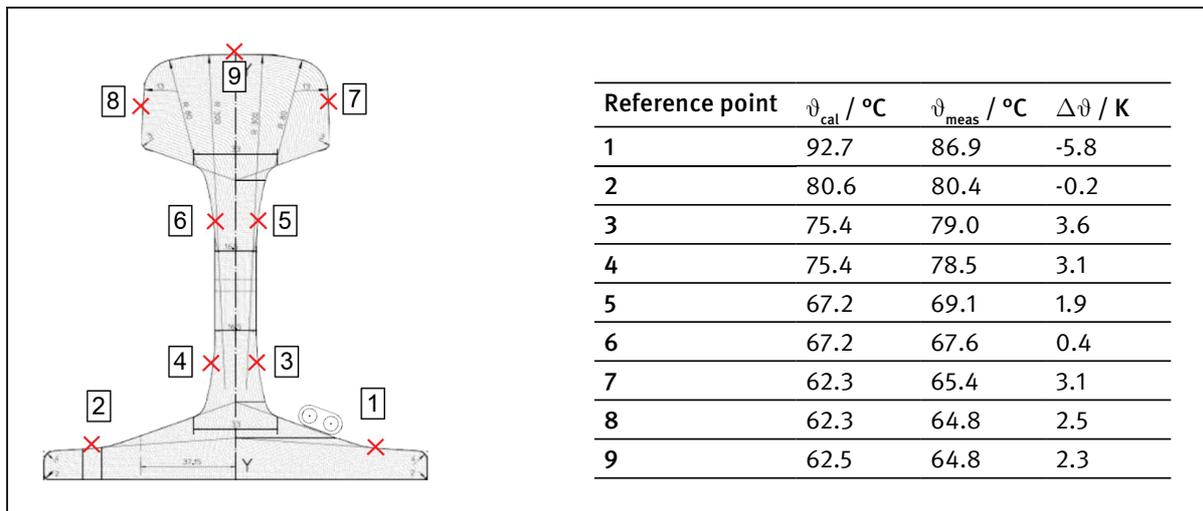
Figure 5 Calculated and measured temperatures at different reference points on the rail
