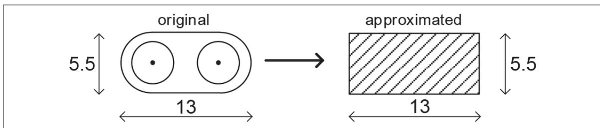
**Figure 1** Original and approximated cross section of the heating rod
