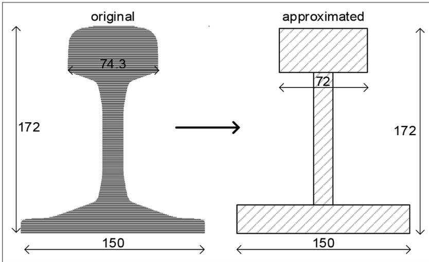
Figure 2 Original and approximated cross section of the stock rail
