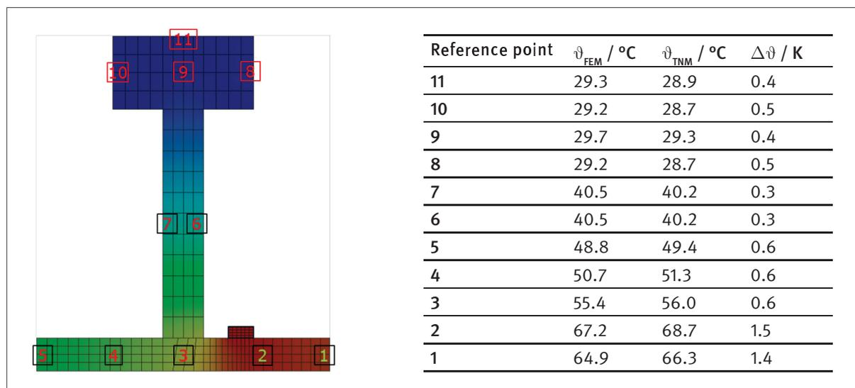
**Figure 4** Heating calculation results by FEM and TNM
