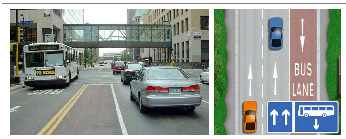
Figure 2 Contraflow bus lane [2]
