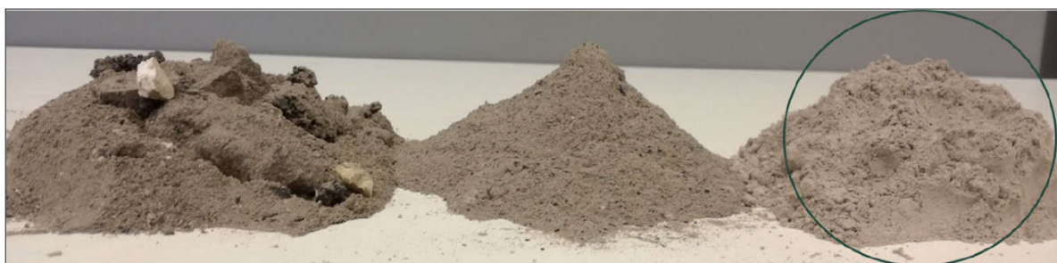
Figure 2 Bioash fractions from Strizivojna Hrast”, left to right: bottom ash, cyclon fly ash, electrofilter fly ash
