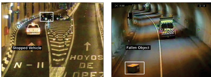
Figure 3 Intelligent tunneling management – Incident situations [13]
