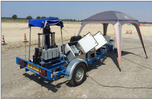
Figure 1 Fast Falling Weight Deflectometer – FFWD – on trial section
