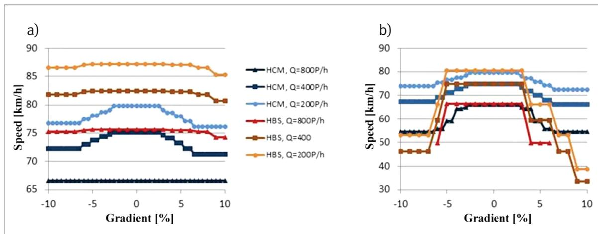
Figure 2 Impact of longitudinal gradient of road's on speed, with heavy vehicles share of traffic at: a) 0 %, b) 15 %
