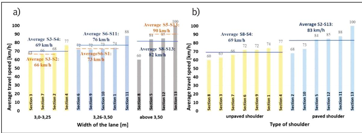
Figure 4 Travel speed on sections: a) of variable lane width, b) of variable type of shoulder
