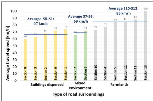
Figure 5 Travel speeds on sections with different types of surroundings
