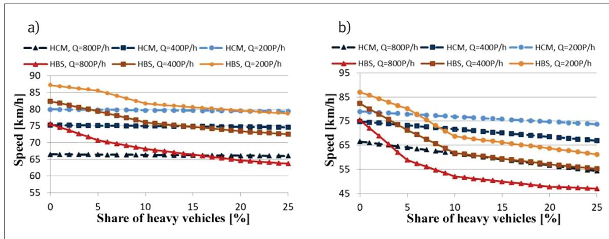
Figure 1 Impact of heavy vehicles on speed: a) flat terrain, b) longitudinal gradient 5 % (P/h – vehicles per hour)
