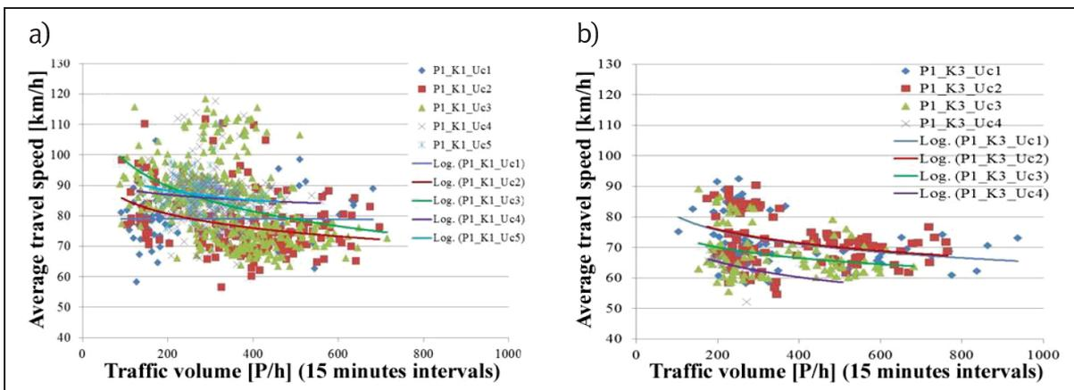
Figure 6 Travel speed depending on traffic volume in the primary direction and share of heavy vehicles for road curvature class/ vertical alignment class in HBS; a) 1/1, b) 3/1. Data from 38 research sites
