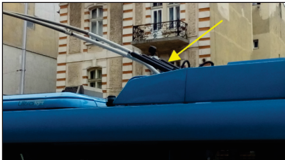
Figure 2 Springs used in trolleybus poles
