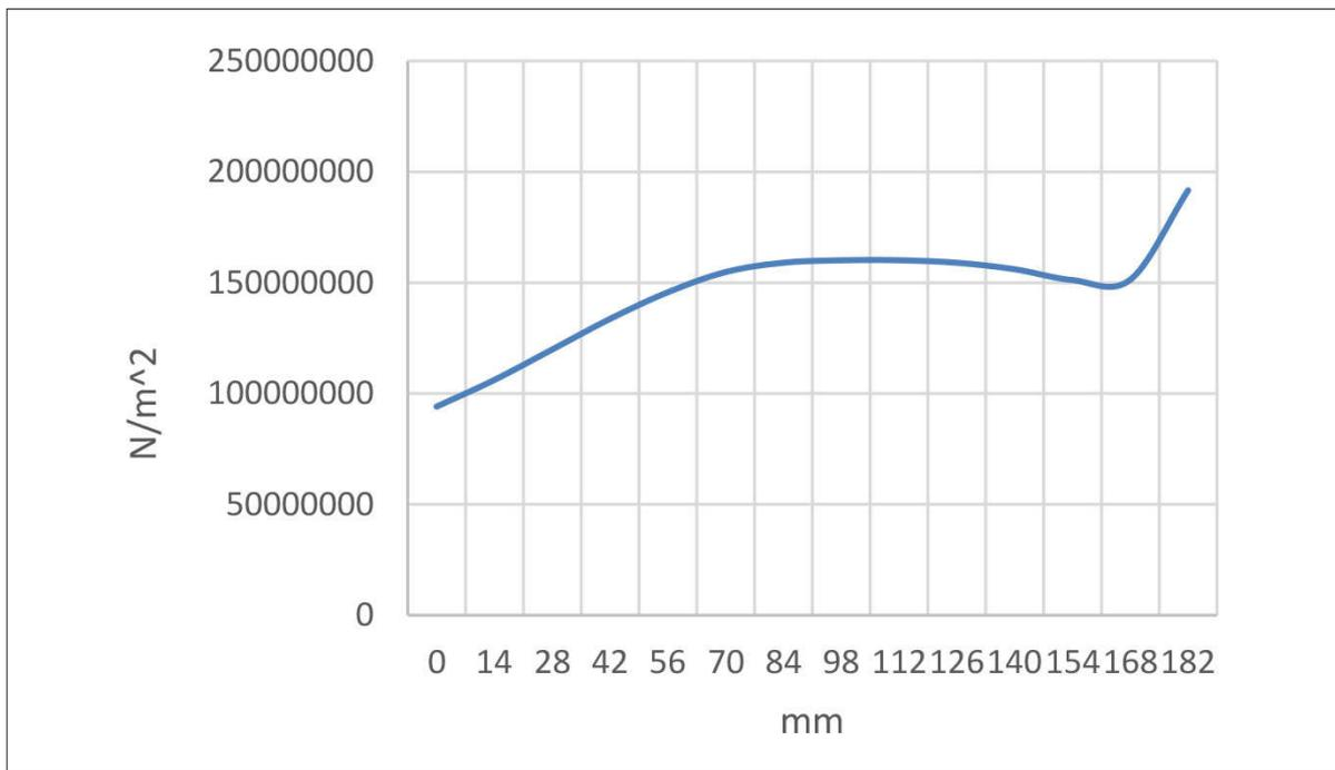
**Figure 3** Distribution of pressure beneath the wheel press fit
