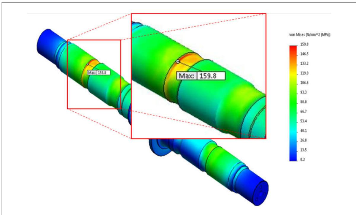
**Figure 4** Calculation result of FEM Analysis
