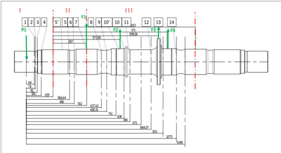
Figure 1 Powered axle of shunting locomotive MDD-04
