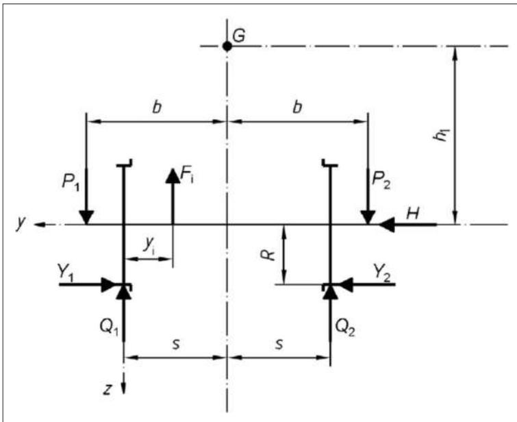
Figure 2 Loads acting on powered axle according to EN 13104 [4]
