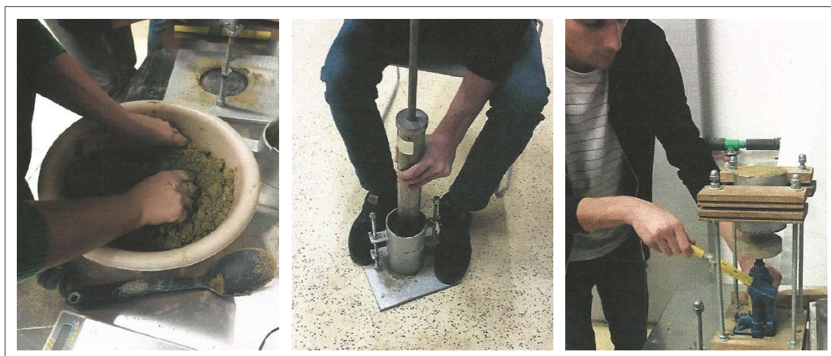
Figure 1 Performing of standard Proctor's test in the laboratory [5]
