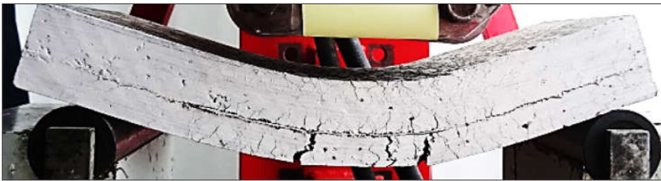
Figure 3 Example of the reinforced specimen after the test
