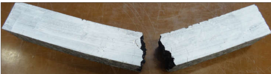
Figure 5 Example of the unreinforced specimen after the test
