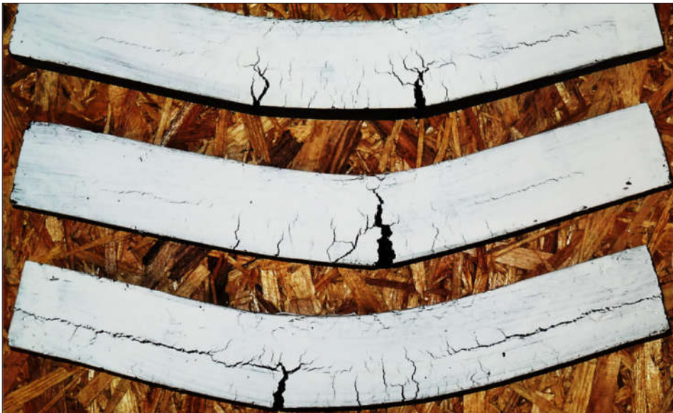
Figure 4 Examples of failure modes of the reinforced specimens
