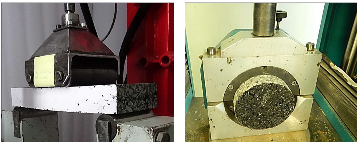
Figure 2 Four-point bending test arrangement (on the left) and Bond condition test (on the right)
