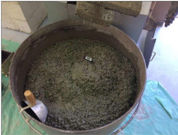
Figure 2 Preparation of a pervious concrete mixture
