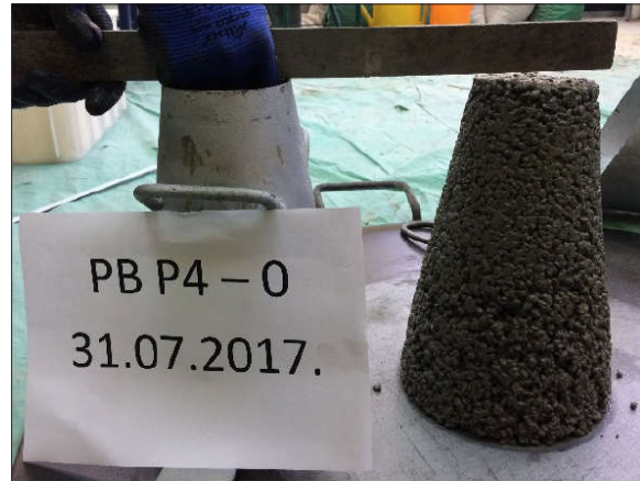
Figure 3 Measurement of consistency by the Slump test
