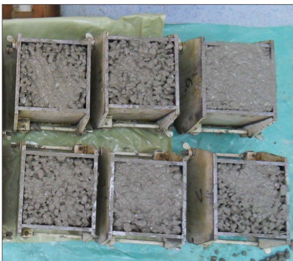
Figure 4 Concrete embedded in molds
