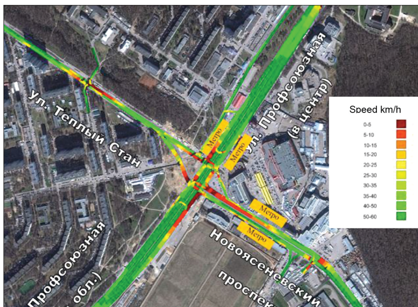
Figure 3 Micro-level (local modeling), including the assessment of individual transport hubs and linear road facilities
