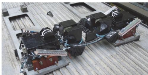
Figure 1 Contactless measurement device for OCL
