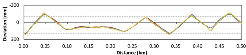
Figure 4 Static stagger of contact wire
