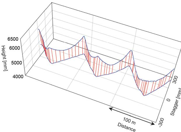
**Figure 5** Measurement result of OCL 3D structure
