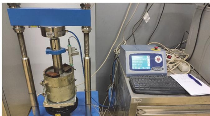
**Figure 2** Examination of California bearing ratio CBR [15]
