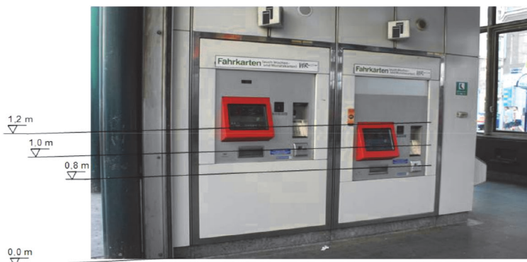
Figure 3 Barrier free ticket machines (ticket machines for everyone) installed in Vienna [10]
