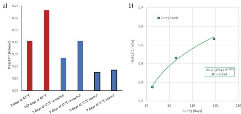
**Figure 2** Evolutions of ITS values during the curing period of: a) sepcimens, b) cores
