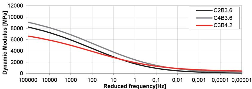
**Figure 1** Master curves for CIR mixtures (PL) for binder (C3B4.2) and base (C2B3.6, C2B3.6) course with similar proportions of binding agents,  $T_{ref} = 20\text{ °C}$
