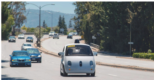
Figure 3 Example of an autonomous vehicle from Waymo LLC without a driver driving on an American road [14]
