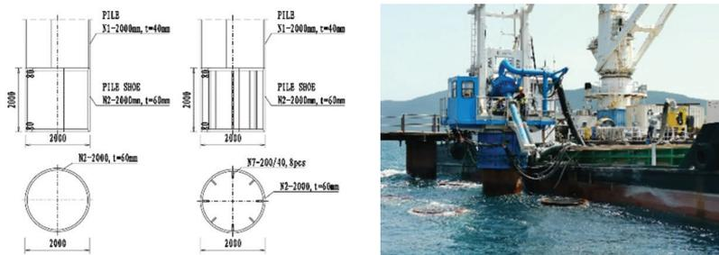
Figure 1 Pile classification and RCD drilling machine
