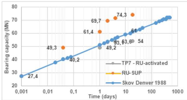
Figure 6 Log-linear long-term pile bearing capacity
