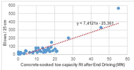
Figure 4 Concrete-socketed pile curve
