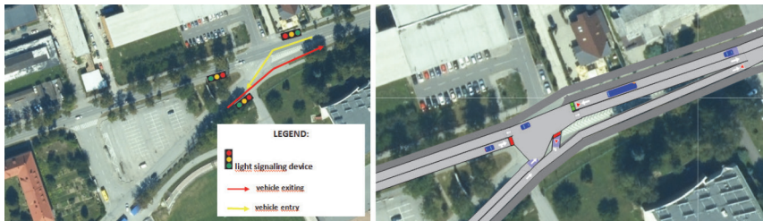
Figure 4 Recommended proposal to change the organization of transport (left panel), the changed state model in Aimsun (right panel) [own study]
